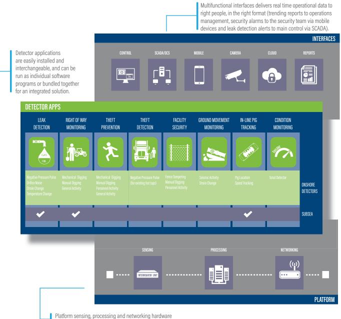
can be easily retrofitted for pipelines with existing fiber optic cables.
